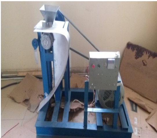
Fig.1: Extruder designed and constructed by the Researcher (A Research Project Sponsored by DUFIL – Indomie Manufacturers, in Conjunction with NOTAP-National Office for Technology Acquisition and Promotion)
